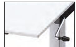
**Gas spring height adjustment.** Ideal force adjustment using the crank handle for individual setting of the table’s live load of up to +50 kg. Benefits: fast and intuitive adjustment, not dependent on power sources, no costs for stand-by mode and maintenance, no CO<sub>2</sub> emissions due to currentless operation, low noise generation.
