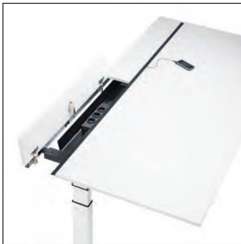
**Elegant.** Functional and aesthetically pleasing: the continuous and two-part electrical connection flap renders the cable tray invisible yet still allows easy and convenient access to power and data connections as and when needed. The brushes make it possible to supply cables to any point.
